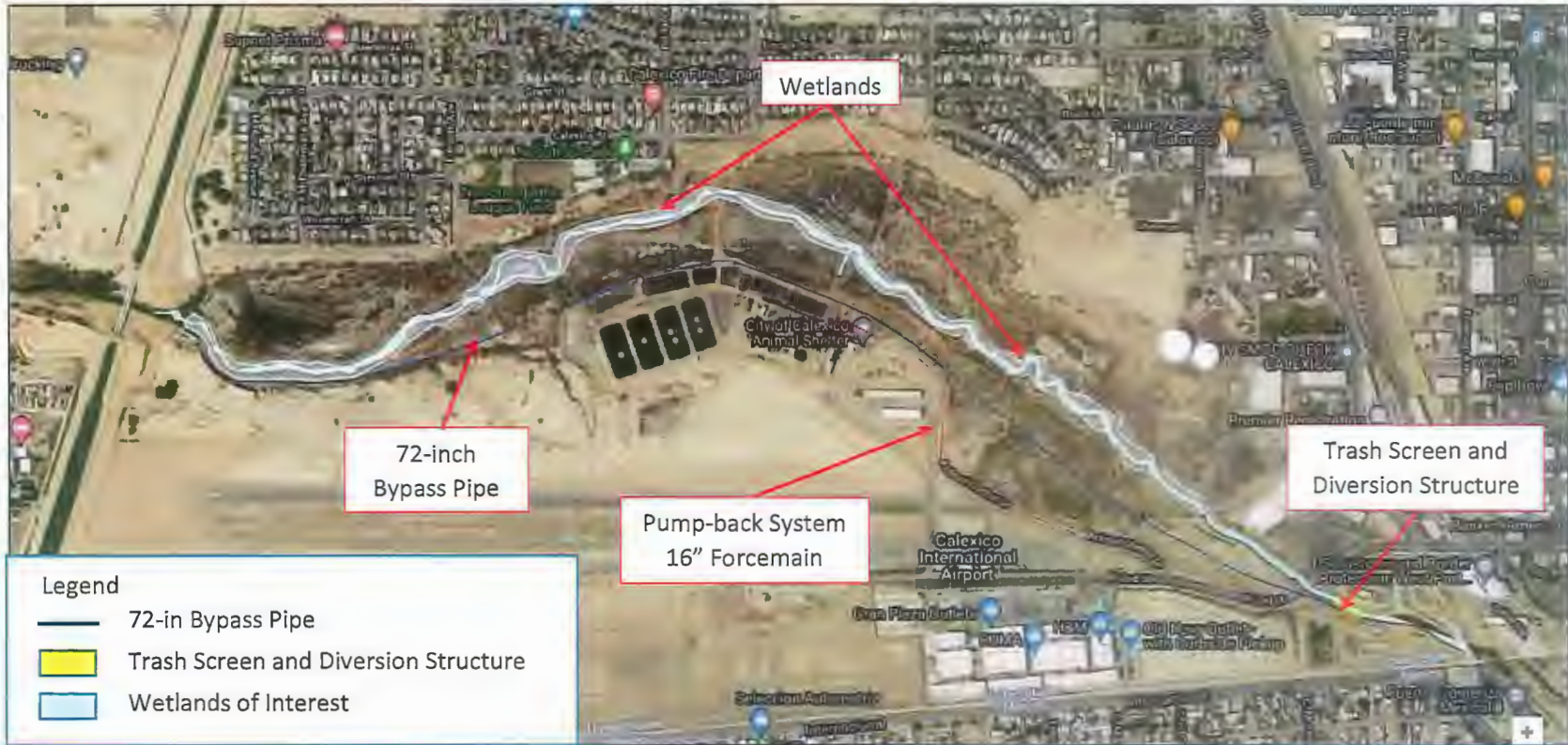
Figure 2 – Project Site and Main Components
